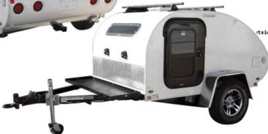
2" Ball Hitch - 7 Pin Power Connector - 1200 lb - 6 ft Cabin (11 ft total length)
